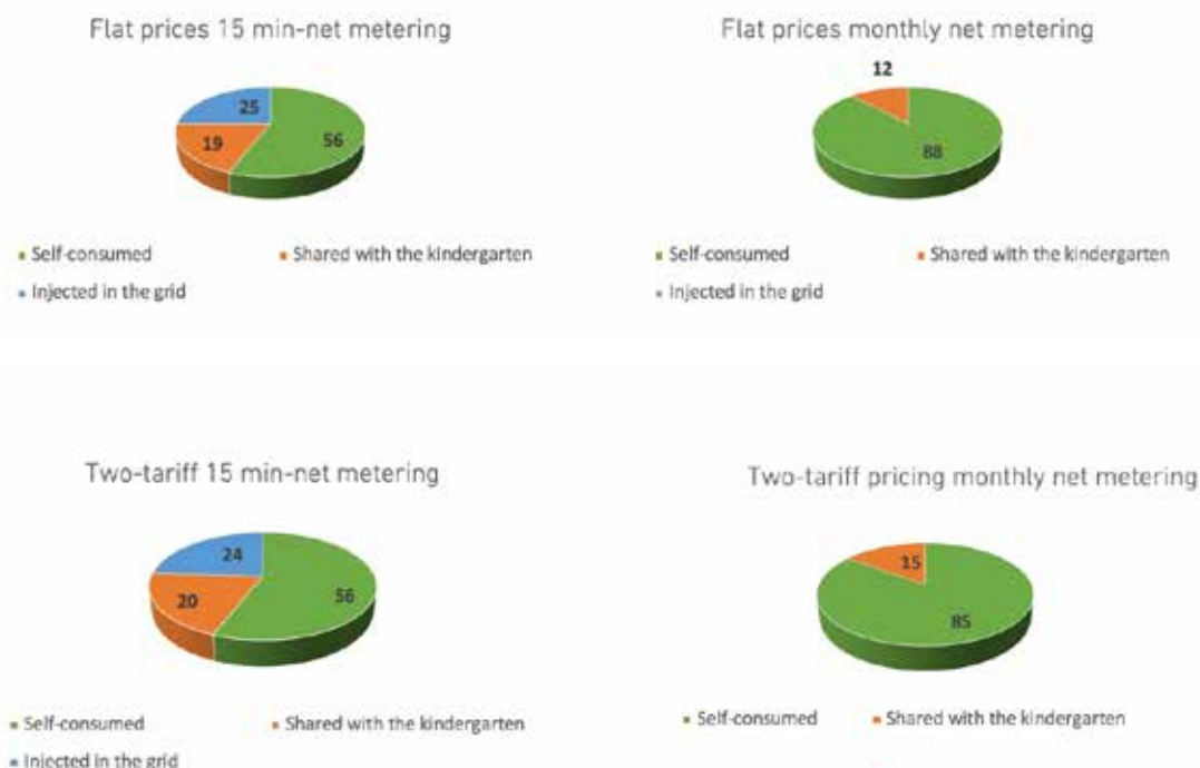
Figure 5. Use of PV production in different net-metering approaches
